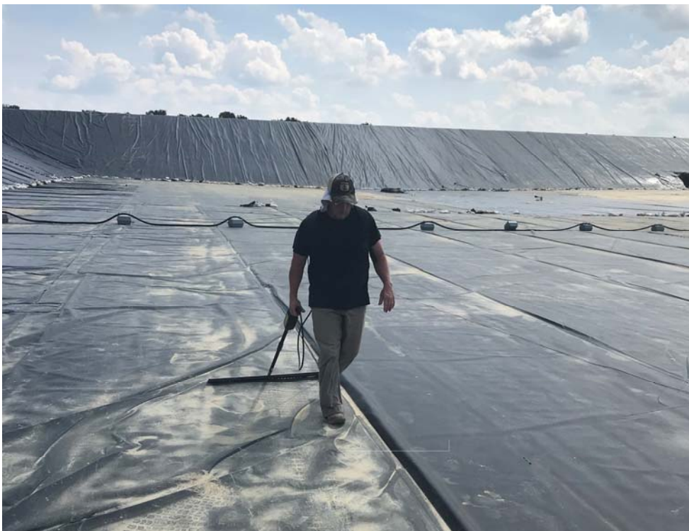
Photograph 2: Arc Testing Method in progress, performing ELL in Contract A - Storage Lagoon.
